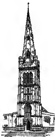
F ST PETER KETTERING, NORTHANTS CASTELLATED ANGLE TURRETS & PARAPET
